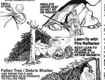
PILE DEBRIS OR SNO ONTO SHELTER FOR ADDED INSULATION
